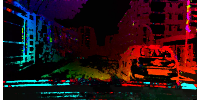
Fig. 3. Example of optical flow between two consecutive frame. The hue of a pixel denotes the direction of the flow in that point, while the intensity encodes its magnitude. A bus and a car can be seen on the left and on the right of the image, respectively.
