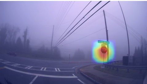
Fig. 5. Saliency map computed from the stop sign detector. When the image contains stop signs, the network focuses its spatial activation in the neighborhood around stop sign positions.
